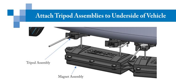
Attach the Tripod Assemblies to the underside of the vehicle directly above where the cord comes out of the top of the magnet assembly.
