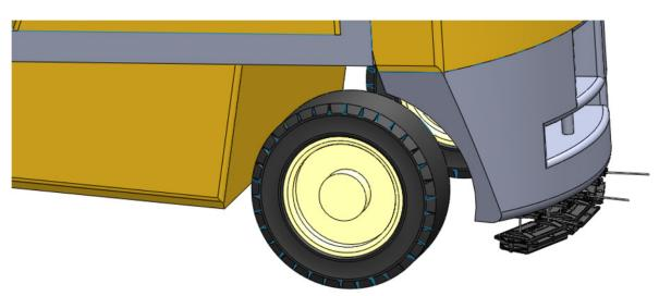
Place the magnet assemblies on the ground underneath the vehicle and arrange so that no part of the magnets will stick out past the edge of the vehicle they are mounted to. Then, wipe off desired area of vehicle where the magnet will be attached to.
