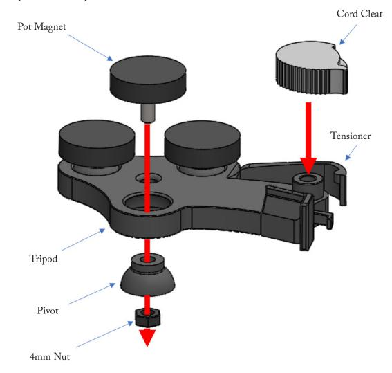
To install the Pot Magnets, place a 4mm nut into the bottom of a Pivot, hold the Pivot with the 4mm nut in the Tripod. Screw the Pot magnet down into the Pivot with nut. Finger tight is ok. Repeat for the other 2 Pot Magnets
