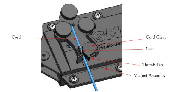
Insert the Cord through the hole in the center of the Pot Magnets. Then place the Cord through the adjustable gap on the left side of the Cord Cleat. Use the Thumb Tab to open the gap to help insert the Cord.
